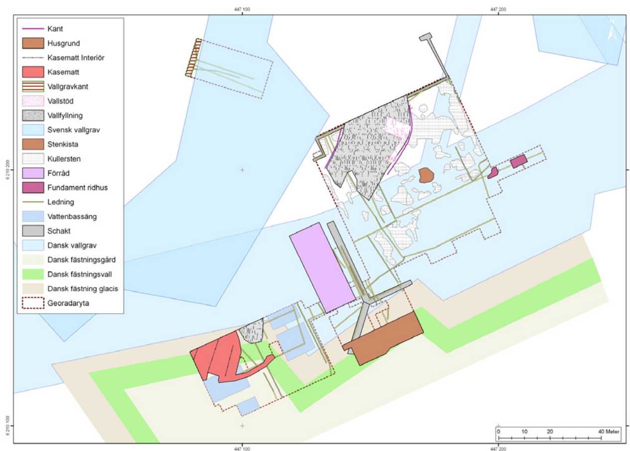
Fig. 2. Several of the areas surveyed with the ground-penetrating radar with the interpretations presented. After L. Winroth & L. Wing, 2020, p. 51.
